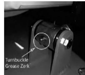
The control arm blocks have grease fittings located on the top of each block. Grease one time a year.
